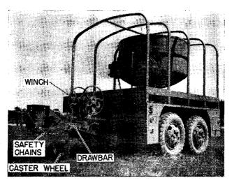
Figure 10. Searchlight trailer M1, loaded (cover removed).
